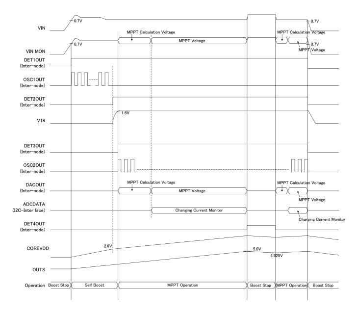
Note) When MPPT operating, it is calculated of MPP each 158mS. (Logosc=30kHz) The amount of the MPP voltage change is 25mV step.
