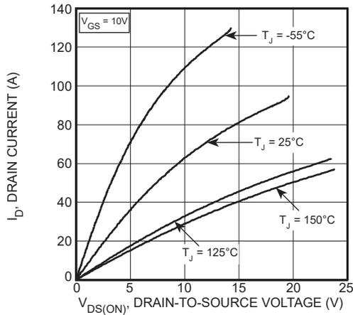
Figure 1, Output Characteristics
