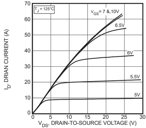
Figure 2, Output Characteristics
