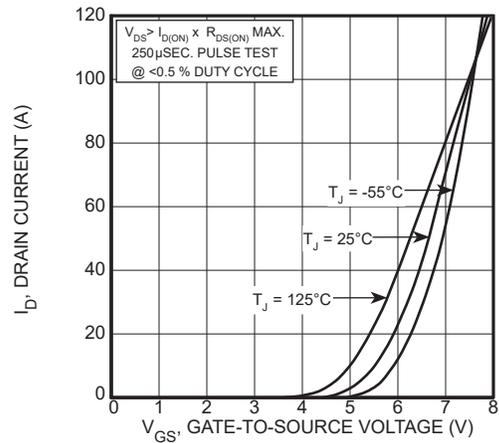
Figure 4, Transfer Characteristics
