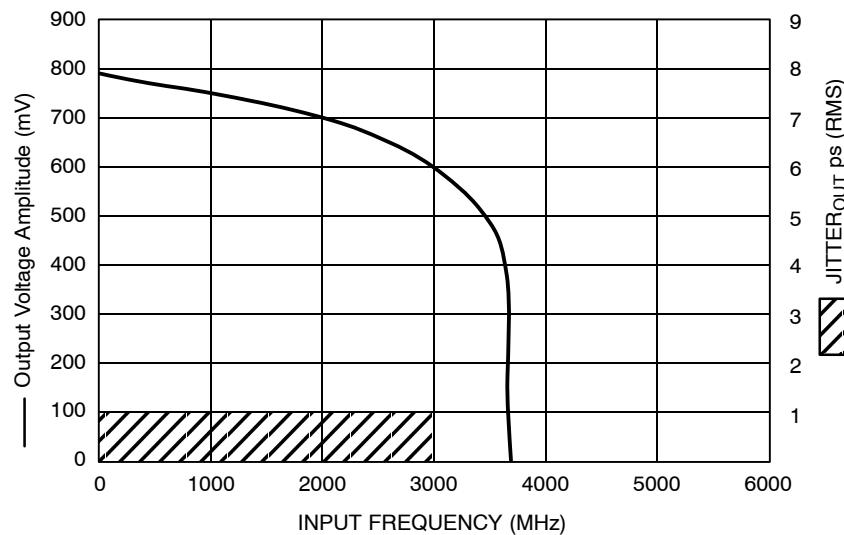
**Figure 4. Output Voltage Amplitude / RMS Jitter vs.
