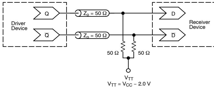
Figure 6. Typical Termination for Output Driver and Device Evaluation
