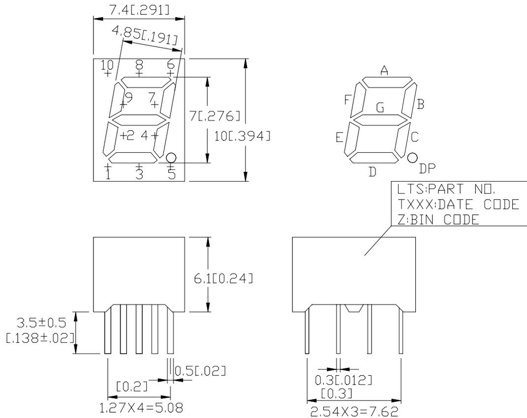
NOTES: All dimensions are in millimeters. Tolerance is  $\pm 0.25$  mm (0.01") unless otherwise noted.
