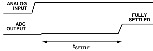
Figure 61. Step Input with Single Cycle Settling
