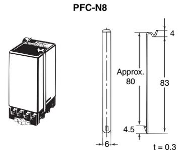
**Note:** PFC-N8 Mounting Bracket (provided with the Level Controller)
