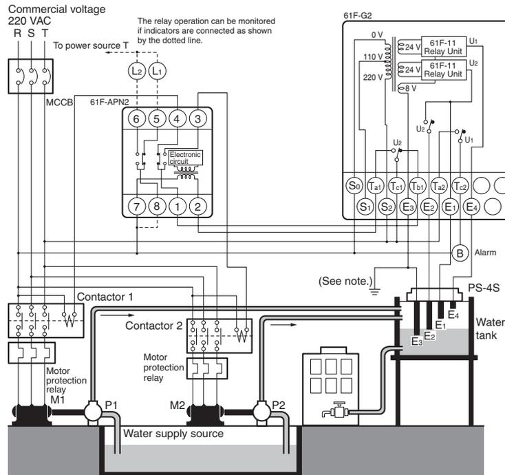
**Note:** Be sure to ground the common Electrode E<sub>3</sub> (the longest Electrode).
