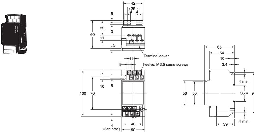
**Note:** Dimensions are with the DIN rail mounting (sliding) bracket attached.
