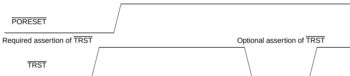
Figure 62. \overline{\text{PORESET}} vs. \overline{\text{TRST}}
