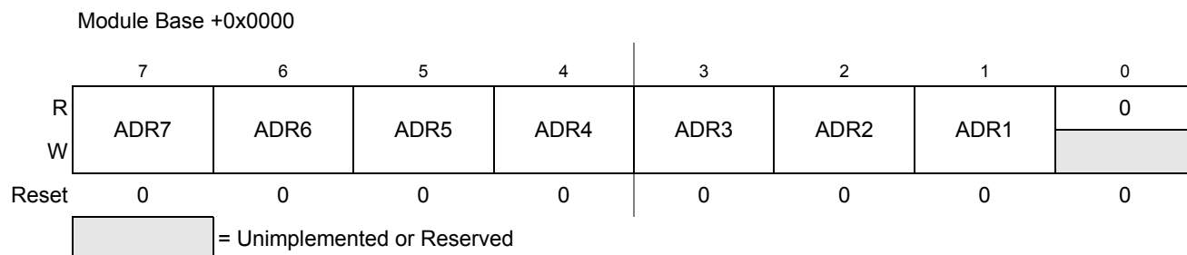
Figure 14-3. IIC Bus Address Register (IBAD)
