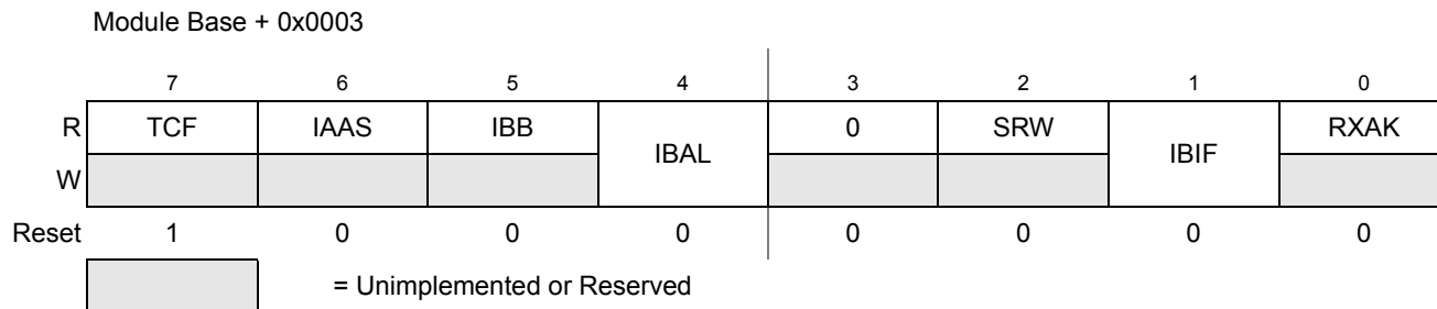
Figure 14-7. IIC Bus Status Register (IBSR)
