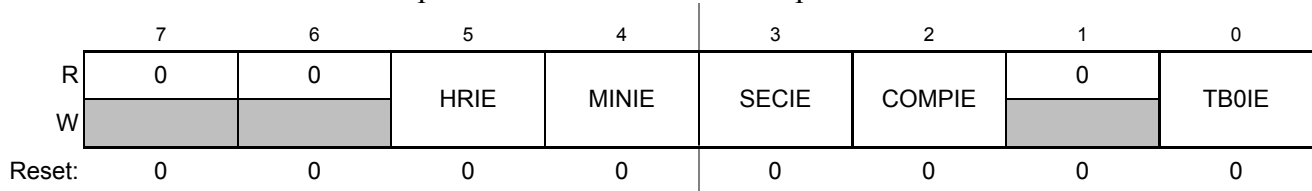
Figure 18-5. RTC Control Register 4 (RTCCTL4)
