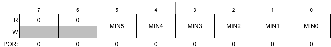
Figure 18-11. Minute Register (MINR)
