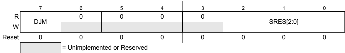
Figure 10-8. ADC Format Register (ADCFMT)
