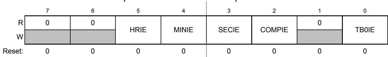
Figure 18-5. RTC Control Register 4 (RTCCTL4)
