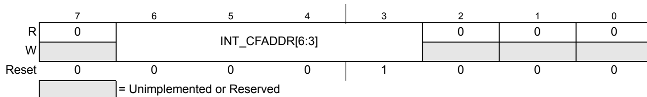
Figure 4-4. Interrupt Configuration Address Register (INT_CFADDR)
