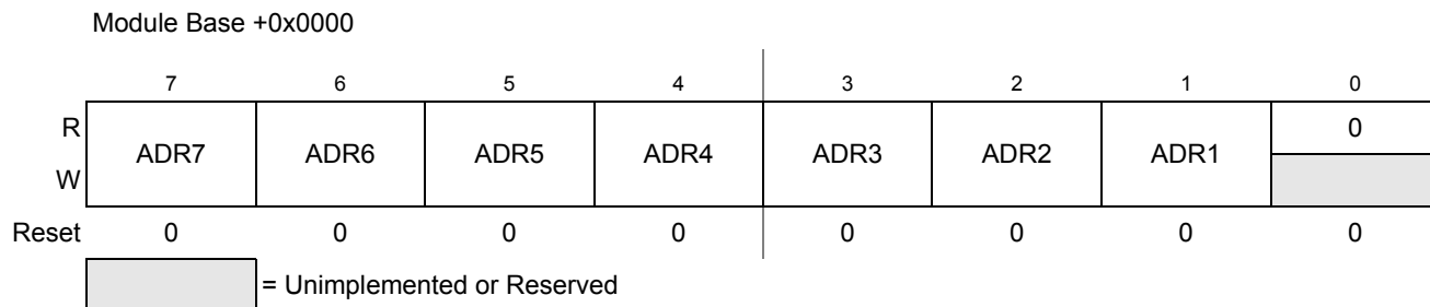
Figure 14-3. IIC Bus Address Register (IBAD)
