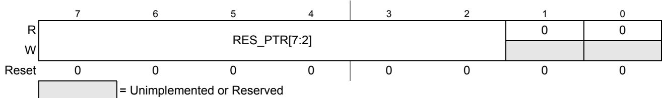
Figure 10-25. ADC Result Base Pointer Registers (ADCRBP_0, ADCRBP_1, ADCRBP_2)
