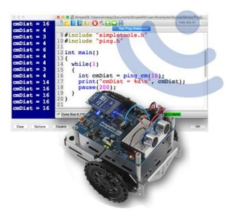
Program the Propeller Activity Board WX over Wi-Fi with the DIP module, and see its remote sensor data display on your computer in real time. This is especially useful when preparing for robot contests because your ActivityBot can roam in a maze and transmit sensor data to the SimpleIDE Terminal without the USB tether. Reprogram it without ever removing it from the maze!
