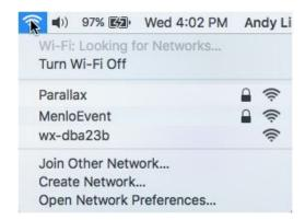
Later, if you have configured your Wi-Fi module to reside on another network, you can make it reappear as an access point by rapidly grounding and releasing the /PGM pin four times. If your Wi-Fi module is in an Activity Board WX, this can be done by pressing and releasing the RST button rapidly, four times. In a breadboard, a pushbutton with one terminal connected to GND and the other to /PGM is convenient.
