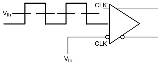
Figure 5. Differential Input Driven Single-Ended ( $V_{th} = V_{REFAC}$ )
