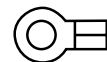
Small Ring for Attaching Receptacle Covers to a Panel with a Screw
