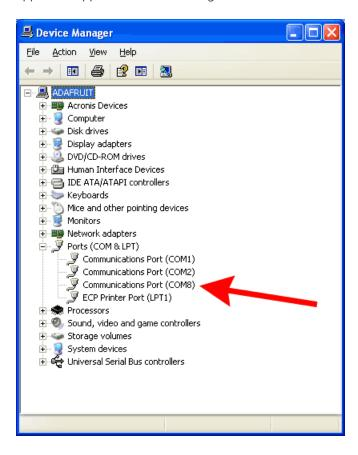
For mac/linux, once you have plugged in the cable, run **dmesg** to see what the name of the port is, probably something like /dev/cu.usbmodem-XXXX or similar. You can also type Is /dev/cu.\* into a Termnal window and see what items appear/disappear when the cable is connected and unplugged.
