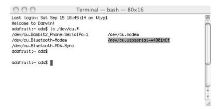
Now that the port is known, you can use your favorite terminal program to connect. For this example, we'll use the basic terminal built into Arduino. The only downside of the serial port monitor is that you can only send a full string at a time and there's a new line at the end. If you are using a more powerful monitor such as CoolTerm (mac) or RealTerm (Windows) you can watch as each character is entered
