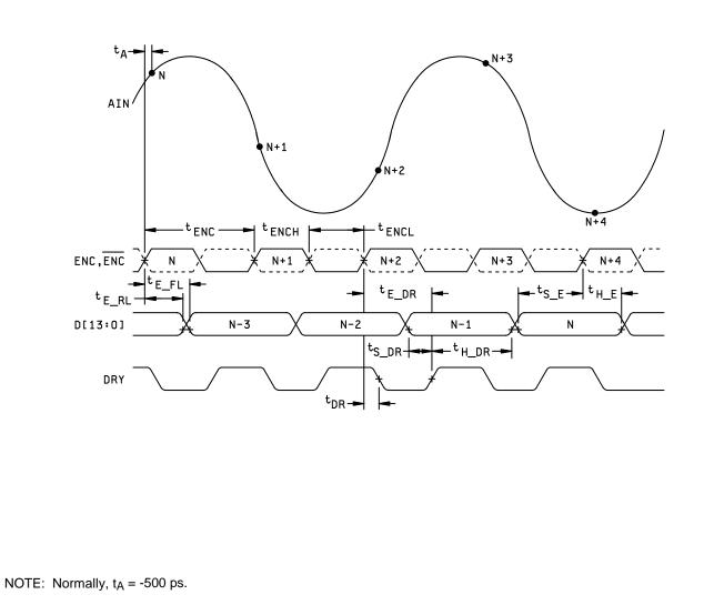
FIGURE 3. Timing waveforms.
