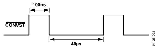
Figure 21. \overline{\text{CONVST}} When Temperature Channel Selected
