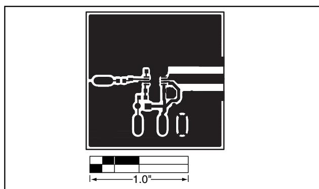
Figure 3. MAX2750/MAX2751/MAX2752 EV Kits PC Board Layout—Component Side
