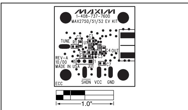
Figure 2. MAX2750/MAX2751/MAX2752 EV Kits Component Placement Guide—Component Side
