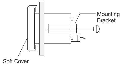
**Note:** Be sure to use the Water-resistive Soft Front Cover and mounting bracket together.
