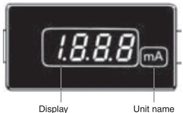
Select the decimal position with the slide switch under the cover on the front panel (signal monitor only).
