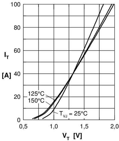
Fig. 1 Forward characteristics
