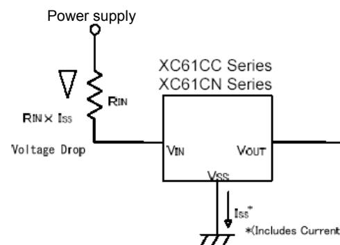
Figure 3: Oscillation in relation to through current
