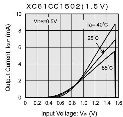
(6) P-ch Driver Output Current vs. Input Voltage
