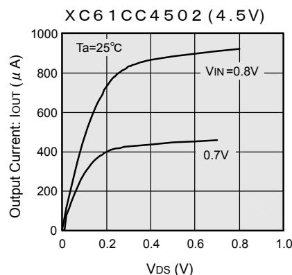
(5) N-ch Driver Output Current vs. Input Voltage
