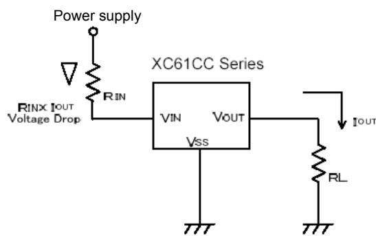
Figure 2: Oscillation in relation to output current
