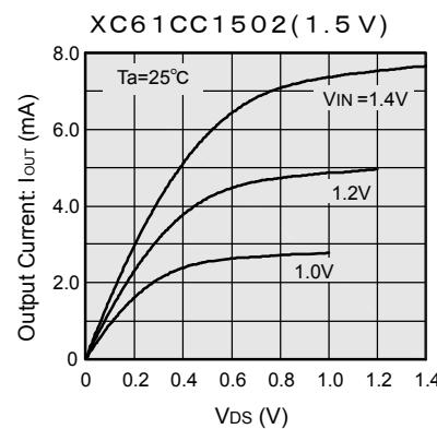
(5) N-ch Driver Output Current vs. Input Voltage
