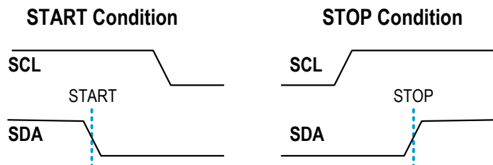
Figure 14. START and STOP Condition Waveform
