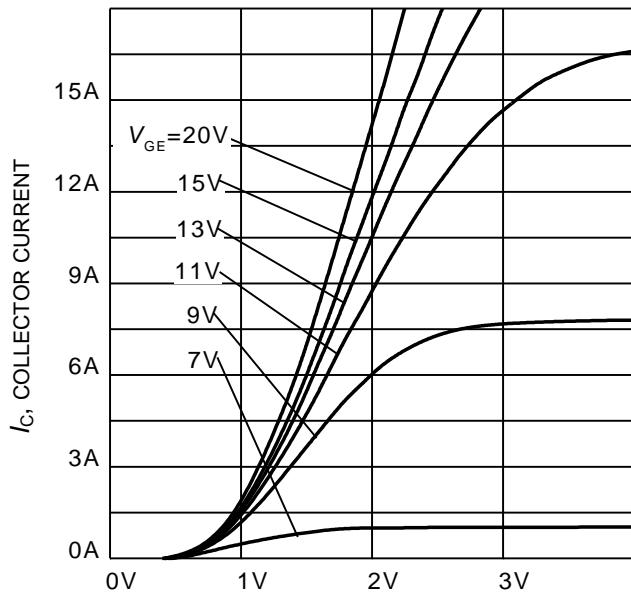
**Figure 5. Typical output characteristic**
