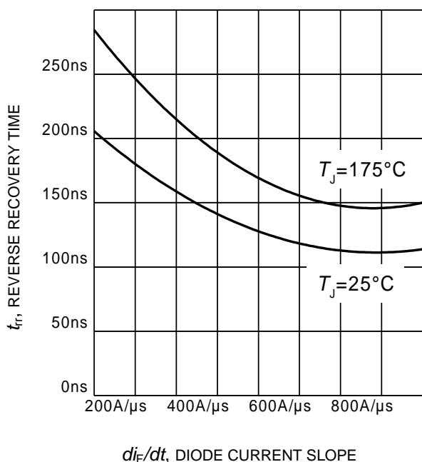
**Figure 23. Typical reverse recovery time as a function of diode current slope**
