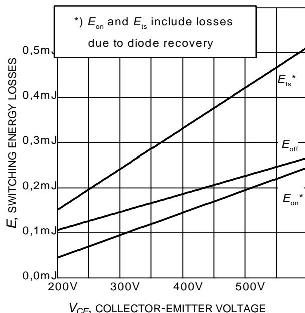
**Figure 16. Typical switching energy losses as a function of collector-emitter voltage**
