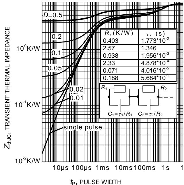
**Figure 22. Diode transient thermal impedance as a function of pulse width**
