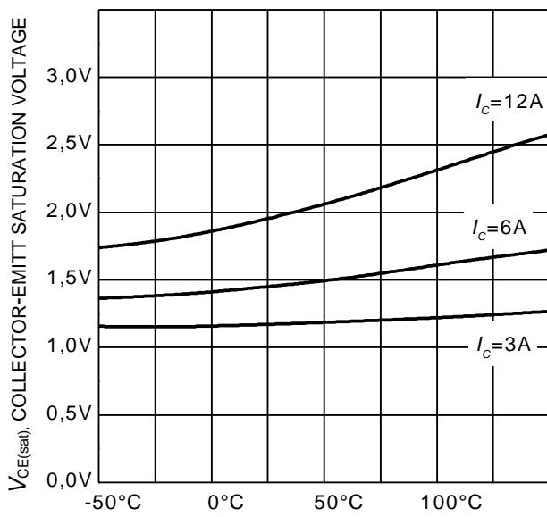
**Figure 8. Typical collector-emitter saturation voltage as a function of junction temperature**
