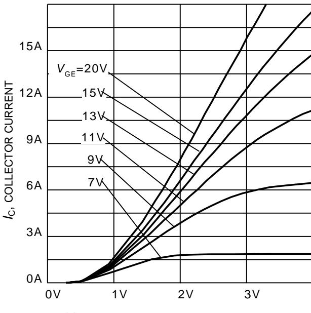
**Figure 6. Typical output characteristic**
