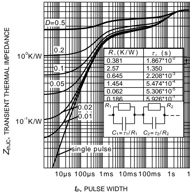
**Figure 21. IGBT transient thermal impedance**
