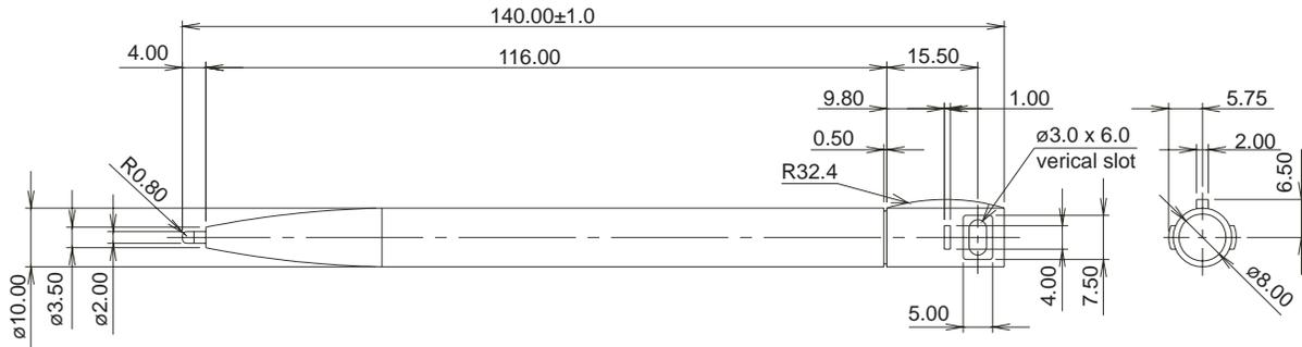
Note: The dimensional tolerance is ±0.5mm unless otherwise specified. Not to scale.
