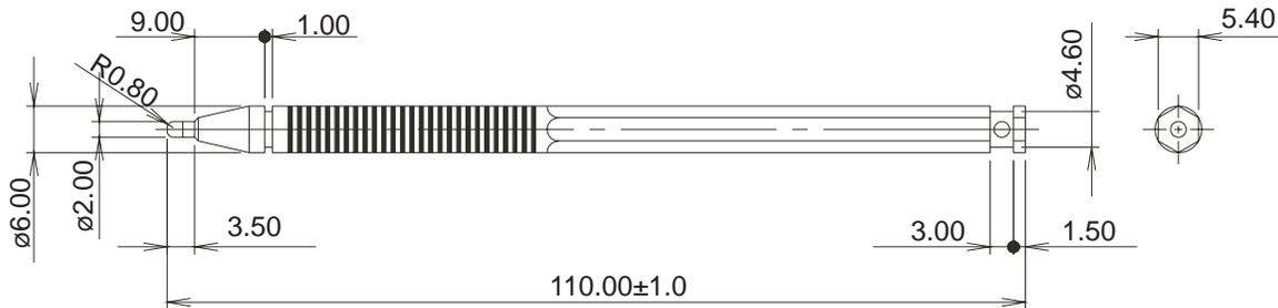
Note: The dimensional tolerance is ±0.5mm unless otherwise specified. Not to scale.
