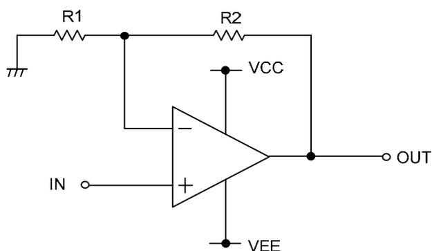
For non-inverting amplifier, IN is amplified by voltage gain decided R1 and R2, and phase is same with IN.
