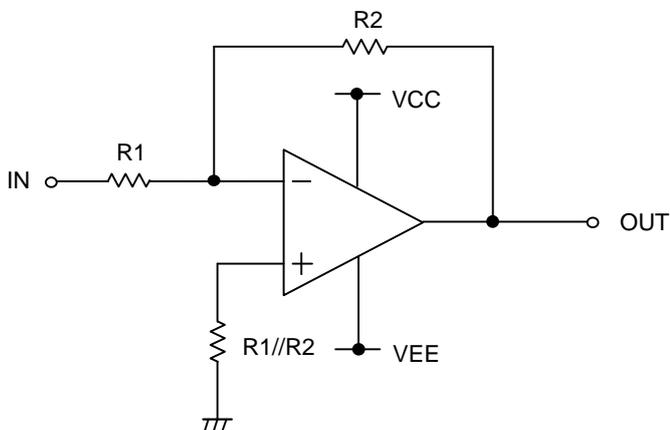
For inverting amplifier, IN is amplified by voltage gain decided R1 and R2, and phase reversed voltage is output.
