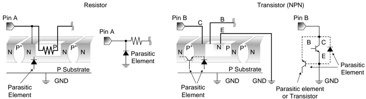
Figure 103. Example of Monolithic IC Structure
