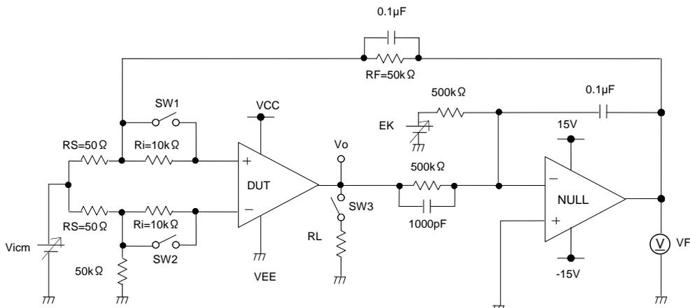
Figure . 98 Test circuit1 (one channel only)
