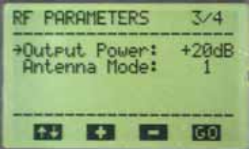
Figure 18. Screen 3: RF Parameters (Antenna Diversity Card Fitted)
