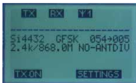
Figure 21. Non-Antenna Diversity Testcard
