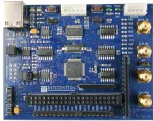
Figure 2. MSC-DBLB2 (Not Included) Testing Platform for controlled Lab Tests (Loadboard)
