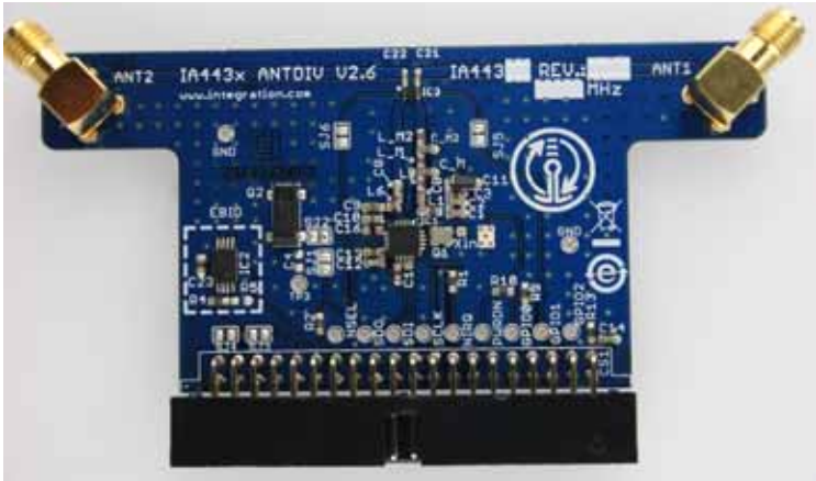
Figure 15. Antenna Diversity Testcard (May be Ordered Separately)
