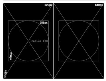
The fbx2 program performs repeated screen captures, scaling it by 50% (providing a smooth 2:1 downsampling in the process) and then copying two squares centered on these regions to the connected SPI screens. For OLED or TFT, the screens are 128x128 pixels, so the sections of the screen copied are 256x256 pixels, and the eyes have a radius of 128 pixels. IPS screens are 240x240 pixels, so the copied sections are 480x480 pixels and the eyes have a radius of 240 pixels.
