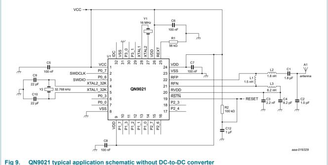
QN9021 typical application schematic without DC-to-DC converter
