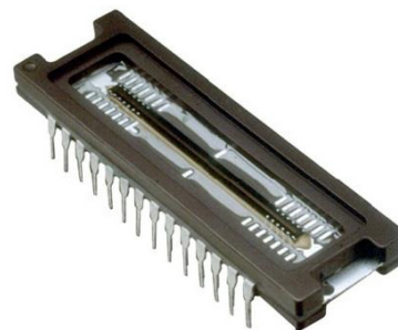
Figure 1. KLI-2113 Linear CCD Image Sensor
