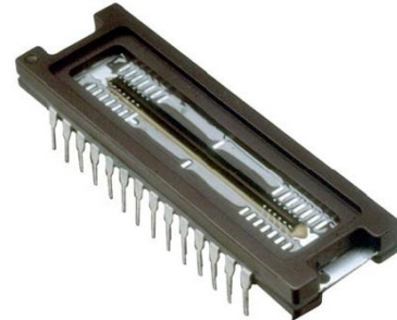
Figure 1. KLI-2113 Linear CCD Image Sensor
