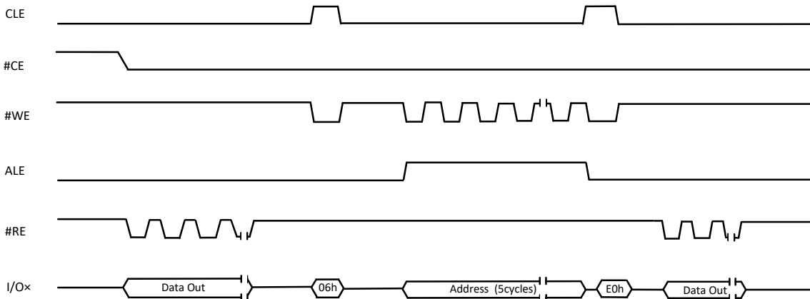
Figure 9-4 Two Plane Random Data Read (06h-E0h) Operation
