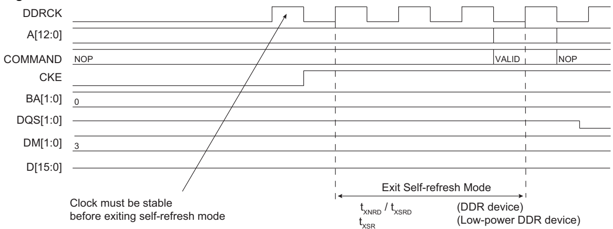
Figure 35-15. Self-refresh Mode Exit
