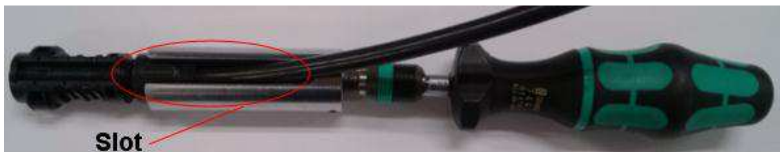
Figure 9 Tightening of the cable screw joint nut
