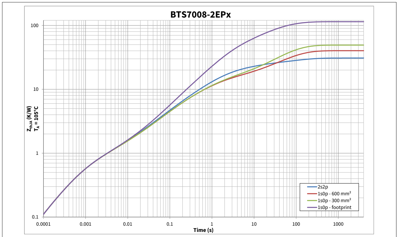
Figure 9 Typical Thermal Impedance. PCB setup according Chapter 4.4.1
