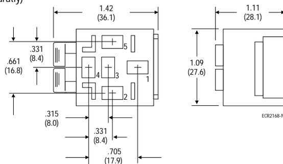
Connectors for VF4/F4; VF7/F7
