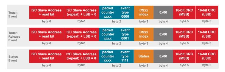
Figure 4.2. I2C Event Buffer Packet Structure
