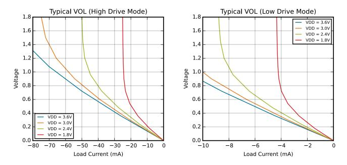
Figure 3.3. Typical  $V_{OL}$  Curves
