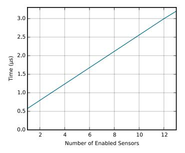
Figure 3.1. Active Mode Processing Time Per Sensor
