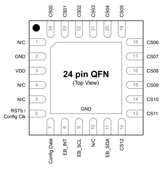
Figure 5.1. CPT213B QFN24 Pinout
