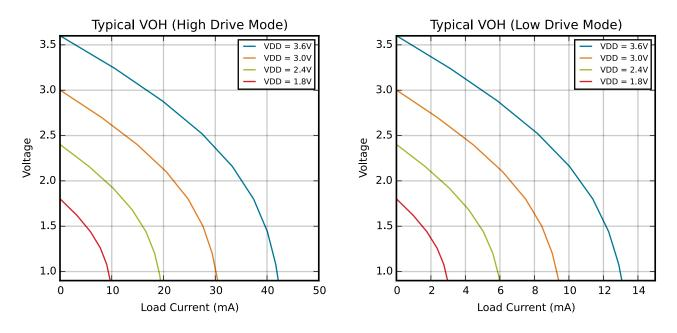
Figure 3.2. Typical V<sub>OH</sub> Curves
