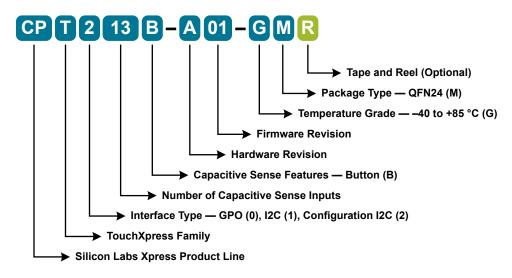
Figure 1.1. CPT213B Part Numbering
