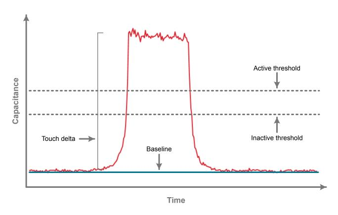
Figure 4.1. Capacitive Sense Data Types
