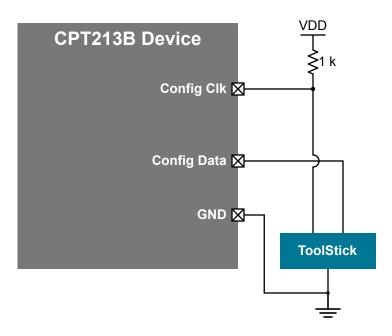
Figure 2.2. Configuration Connection Diagram
