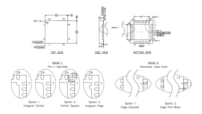
Figure 6.1. QFN24 Package Drawing
