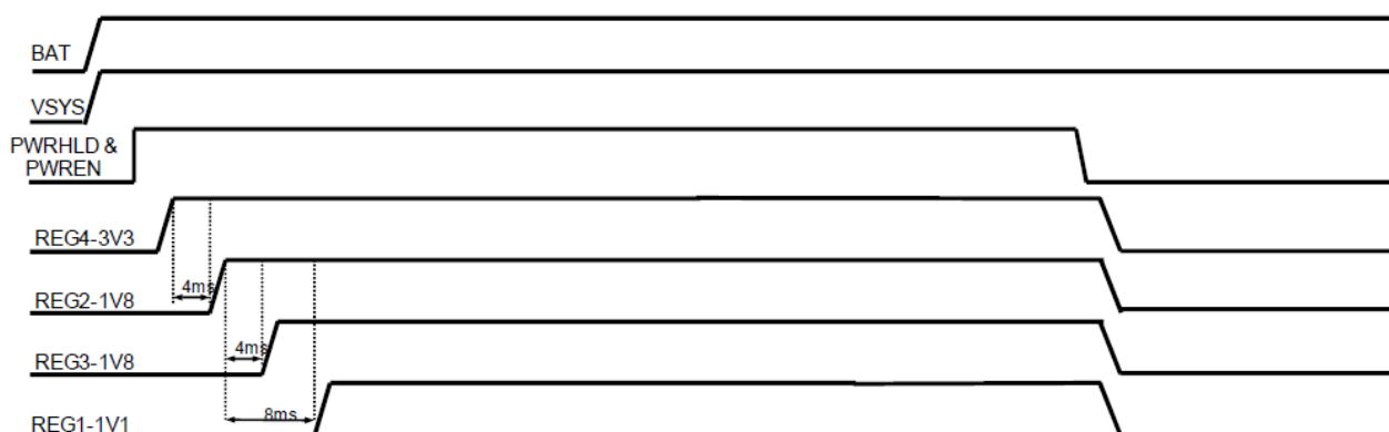
Figure 2: ACT8946AQJ203-T Enable/Disable Sequence
