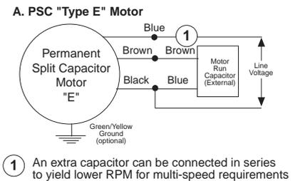
① An extra capacitor can be connected in series to yield lower RPM for multi-speed requirements
