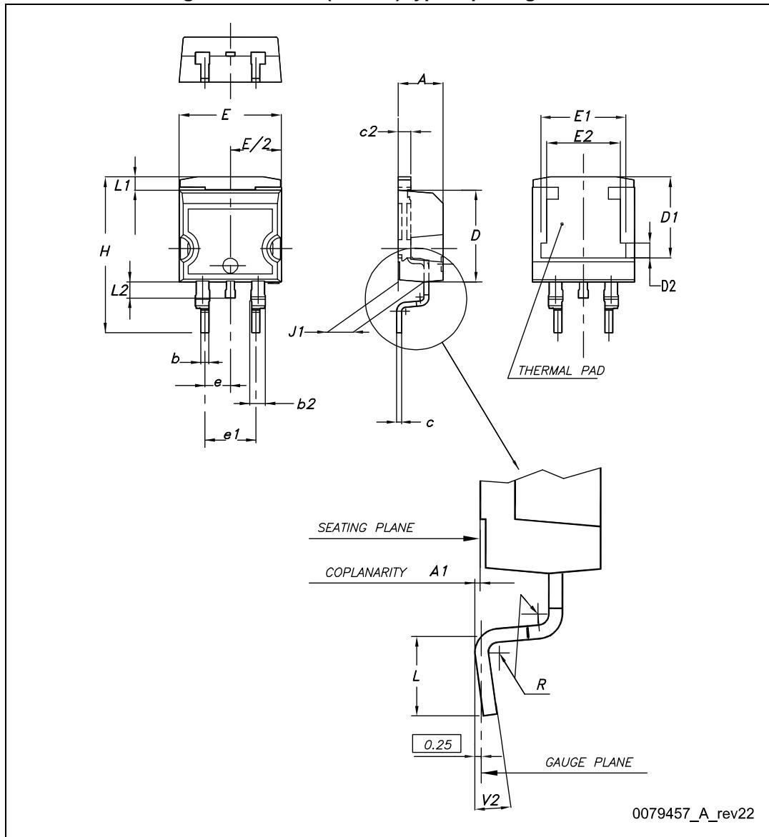
**Table 8. D<sup>2</sup>PAK (TO-263) type A mechanical data**
