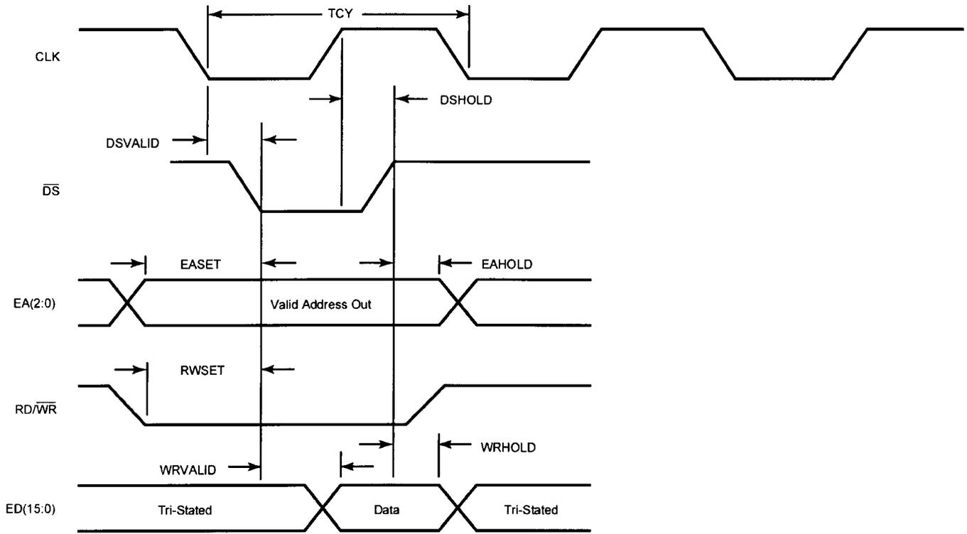
Figure 9. Write Timing
