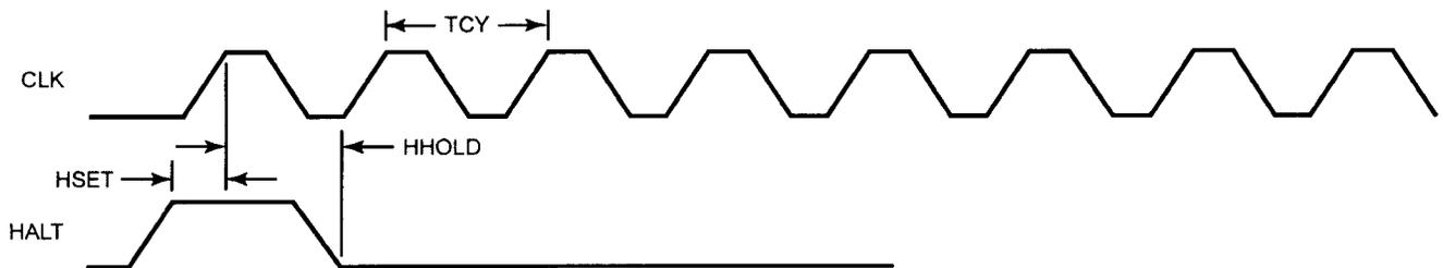
**Figure 12. HALT Timing**
