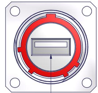
USB A FEEDTHROUGH CONNECTOR GROUNDED TO OUTER SHELL
