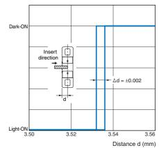
Vcc = 24 V, No. of repetitions: 20, Ta = 25°C Differential distance = 0.025 mm max.
