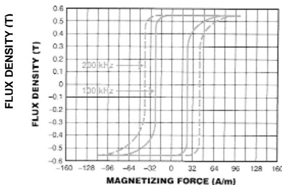
METGLAS® Square Loop magnetic cores are specifically designed to exhibit an extremely square dc Hysteresis loop and high BSAT resulting in the following important benefits:
