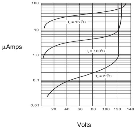
Instantaneous Reverse Leakage Current - MicroAmperes versus
