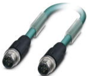
Network cable, Ethernet CAT5, Ethernet CAT5, 4-position, shielded, Plug straight M12, on Plug straight M12, cable length: 6 m
