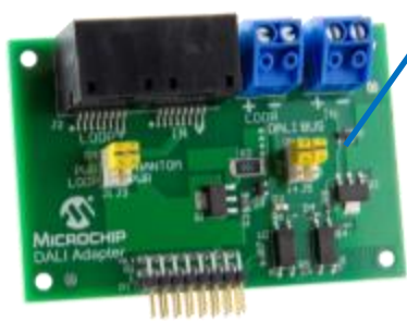
DALI Adapter with 2-wire & RJ45 connections
