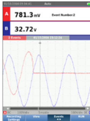
Quickly step through recorded events to identify and troubleshoot intermittent faults.
