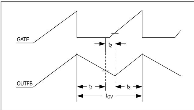
Figure 5. MAX6495/MAX6496/MAX6499 Timing
