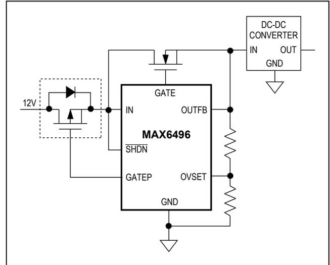
Figure 7. Overvoltage Limiter with Low-Voltage-Drop Reverse-Protection Circuit (MAX6496)
