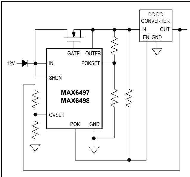
Figure 8. Overvoltage Protection to a DC-DC Converter (MAX6497/MAX6498)
